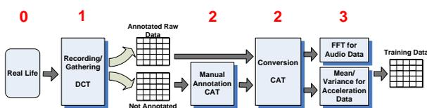
**Figure 5:** Training Data Gain using DCT, CAT and Feature Extraction
