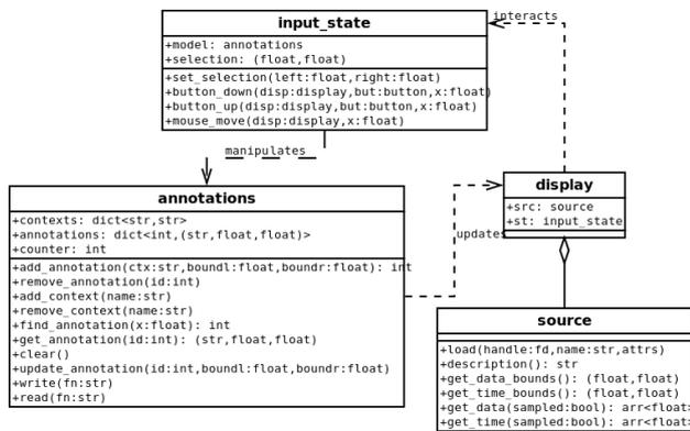
Figure 10: (Partial) class diagram of the CAT
