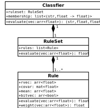
**Figure 4:** Class diagram of the python rule engine
