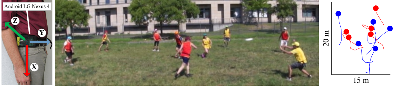
Figure 2. Device Placement (Left) for the Team Sports Group Activity Experiment (Middle) with Relative Subject Locations on the Field (Right)
