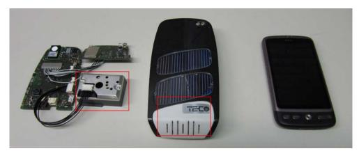
Fig. 1: TECO Envboard: PCBs and Sharp dust sensor (left) and in housing (middle).
