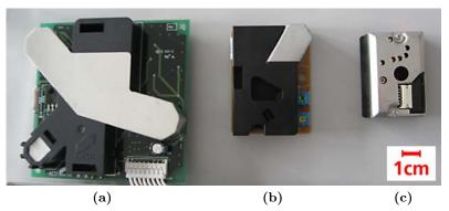
Fig. 3: Particulate matter sensors: AES-1 (a), DSM501A (b), and GP2Y1010 (c).
