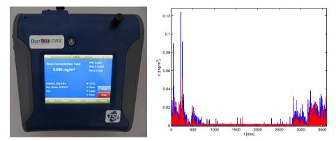
**Fig. 4:** Left: the TSI 8533 DustTrak DRX reference aerosol monitor. Right: data from one of the dust sensors (red curve) and the DustTrak (blue curve) in  $\frac{mg}{m^3}$ .
