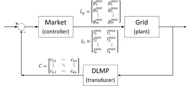
Fig. 3. A control loop for real-time interaction between the power market and grid
