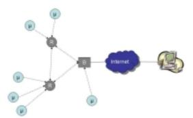
Figure 1. System Architecture with uPart end nodes (µ), router nodes (R) and bridge nodes (B).
