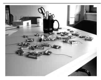
Figure 4. An experiment with over 40 particle computers
